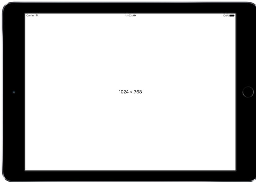
Obviously, the scaling factor is 2. The screen is 9.7 inches in diagonal for a resolution of 132 DPI.
